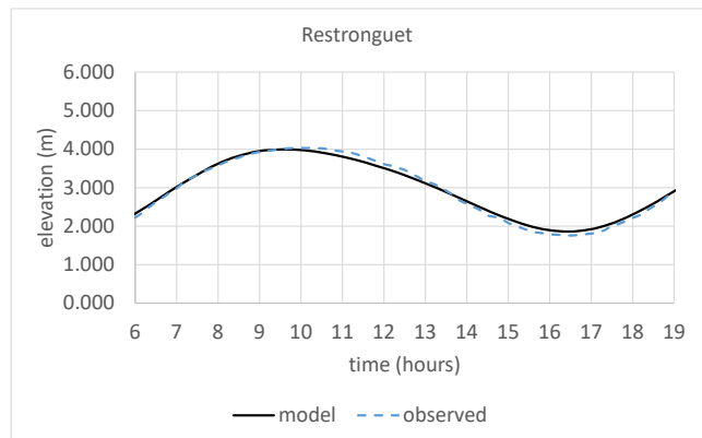
Figure 3.34: Comparison of observed and simulated neap tide water levels at Restronguet
